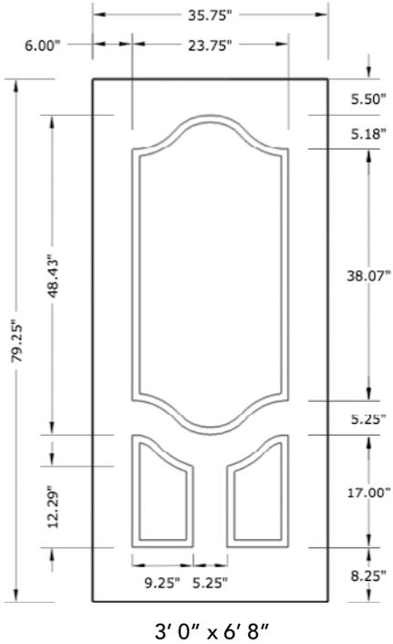
NOTE: BY REQUEST, DOOR HEIGHT COMES IN VARYING DIMENSIONS TO A MINIMUM OF 79". EXCESS WILL BE TAKEN FROM BOTTOM RAIL. ALL OTHER DIMENSIONS WILL REMAIN THE SAME.
